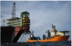
External Turret Production (ETP) for FPSO
