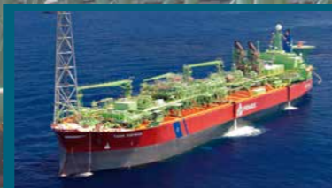
YUUM K'AK'NÁAB (2007) - the world's largest converted FPSO with a throughput capacity of 600,000 bbl per day, operating for Pemex in Mexico
