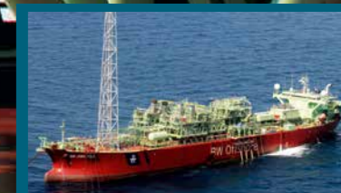
BW JOKO TOLE (2012) - gas compression capacity of 340 mmscfpd, operating for KEI in Indonesia
