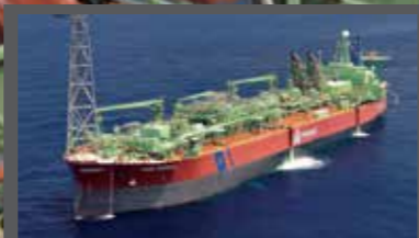
YÙUM K'AK'NÁAB (2007) - the world's largest converted FPSO with a throughput capacity of 600,000 bbl per day, operating for Pemex in Mexico.
