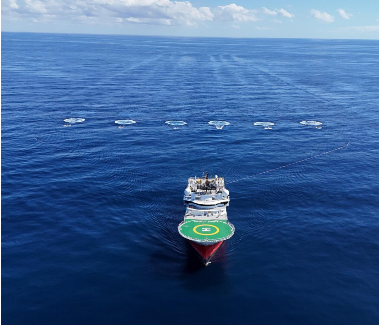
Hexa source configuration testing with the Sanco Swift in the Gulf of America.
