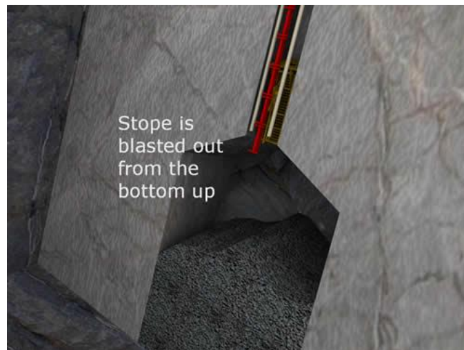
Figure 16-5 RAM Ore Removal
