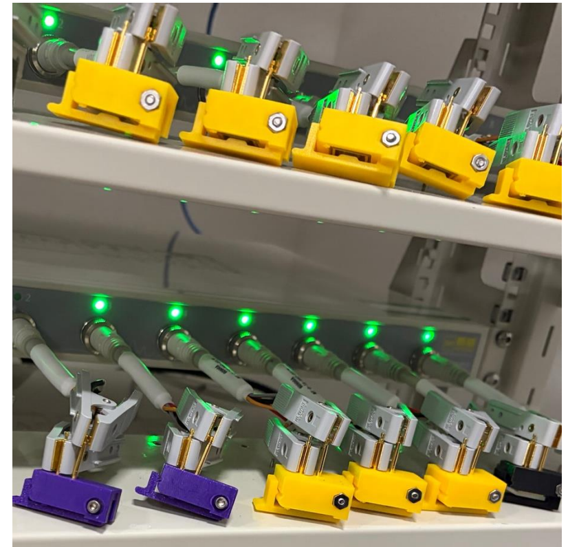
↑ Single layer Ribbon Ceramic cells currently on test at Ensurge; encapsulation enables controlled-environment cycling and accelerates throughput from initiation to data
