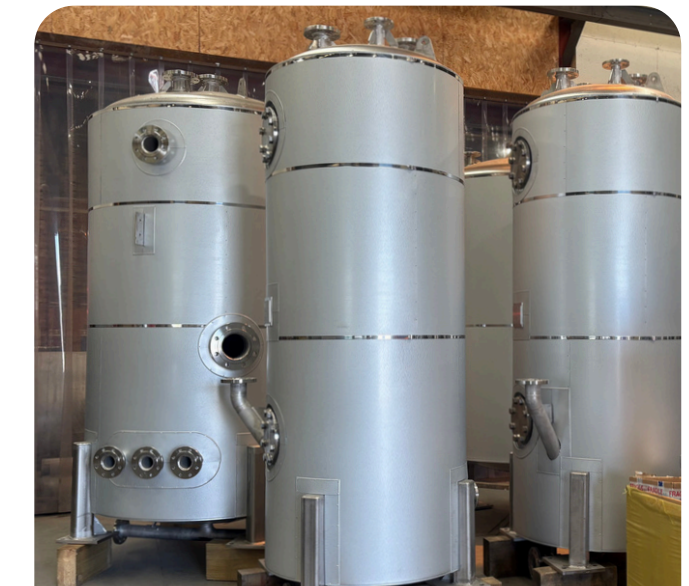
THP pressure vessels for the project in Santiago de Compostela, Spain, awaiting shipment at Cambi's workshop
