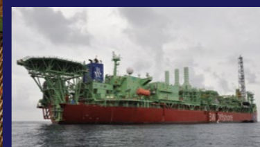
BW PIONEER (2012) - the world's deepest producing FPSO, operating at 2,500 meters in the US GOM for Petrobras.
