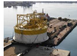
Buoy Turret Loading (BTL) for Shuttle Tankers
